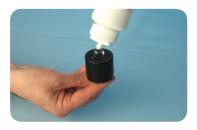
Place ultrasound Transducer through Transducer holder. Ensure cable is routed through cut out on cap and secure by closing cap.
