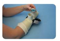
2. Hold Transducer and place a small amount of Transducer gel on the Transducer face. Approximately 1.5cm diameter.
