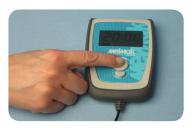
5. Remove Transducer head from treatment site. Clean gel from Transducer head, strap and skin with a soft cloth.
