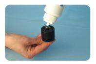
3. Place ultrasound Transducer through Transducer holder. Ensure cable is routed through cut out on cap and secure by closing cap. Ultrasound gel must be touching the skin. Close cap to secure.
