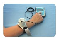
The spring mechanism on the cap provides light pressure to the Transducer. It ensures good contact to the gel and skin over the treatment area for ultrasound transmission.
